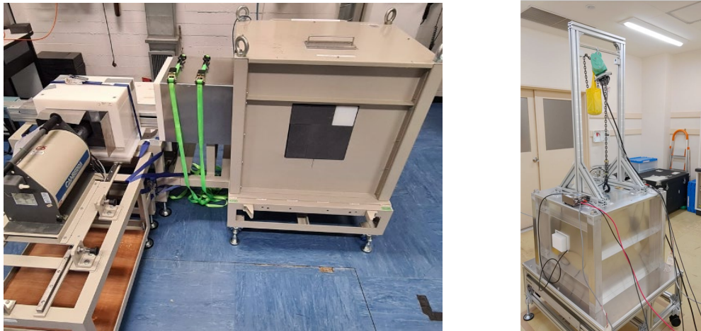
Figure 3. ISCN Delayed Gamma-ray Test Spectrometer in PERLA (left) and Delayed Gamma-ray Demonstration Irradiator in ISCN lab JRR-3L (right).
